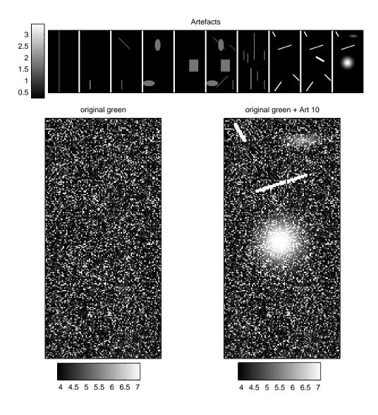
Figure 4.4: Top row: Ten sets of artificial artefacts (we label them  $1, \ldots, 10$  from left to right) to be added to a microarray data slide. Bottom row: the original slide to which artefacts are added and the result of adding the  $10^{\text{th}}$  set of artefacts
