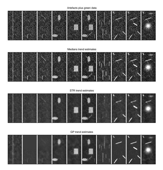
Figure 4.5: Row 1: Data to detrend used as input to the methods. Row 2: Corresponding trends estimated by the Medians algorithm. Row 3: Trends estimated by the STR algorithm. Row 4: Trends estimated by the GP algorithm.
