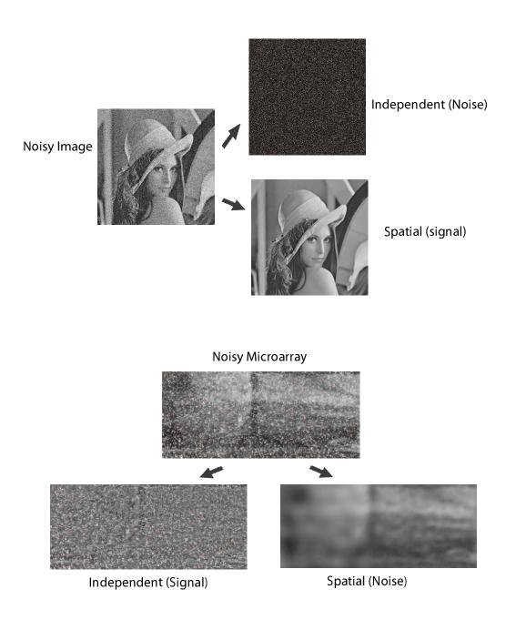
Figure 1.1: The two decomposition problems we will discuss. Top, a noisy image decomposed into noise and the original image. Bottom, a noisy microarray decomposed into probe expression and spatial artefacts.
