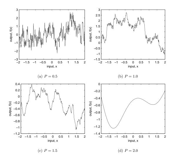
Figure 3.3: One sample function from a Gaussian process with power exponential covariance function, for various values of P (other hyperparameters are fixed at  $\ell = 1$ ,  $\sigma_a = 1$ ).
