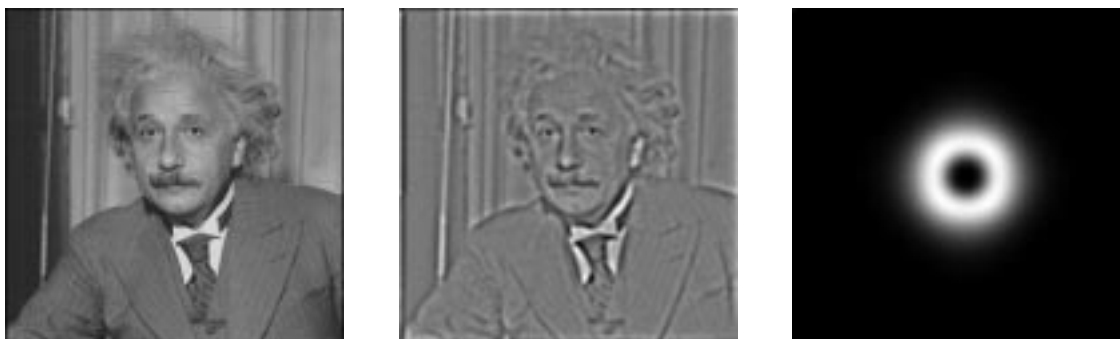
Figure 5: From left to right is the original AI, a band-pass filtered version of AI, and the amplitude spectrum of the filter. This impulse response is defined by the difference of two low-pass filters.
