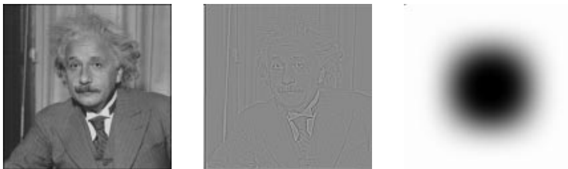
Figure 4: From left to right is the original AI, a high-pass filtered version of AI, and the amplitude spectrum of the filter. This impulse response is defined by \delta[n, m] - h[n, m] where h[n, m] is the separable blurring kernel used in the previous figure.
