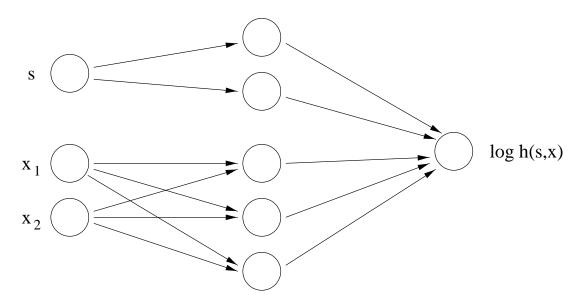
The upper "layer" of two hidden units computes  $\log h_0(s)$ ; the lower layer of three hidden units computes  $\log h_1(x)$ .
