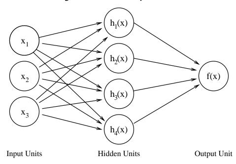
The network takes inputs  $x_1, \ldots, x_I$  and from them computes an output, f(x), using a layer of H hidden units:
